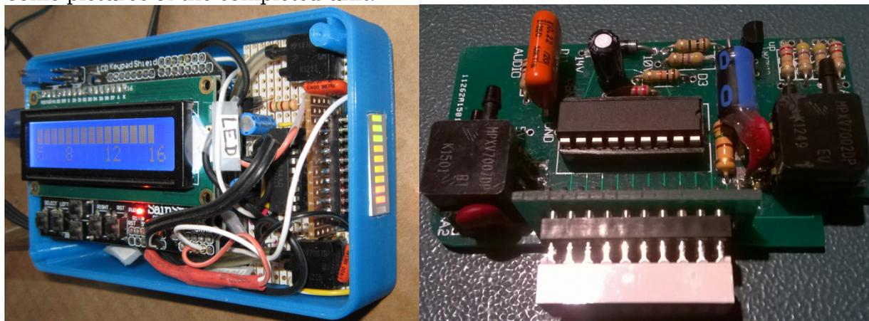
The AoA indicator needs to be calibrated to properly respond to an approaching stall as well as show the current angle of attack on the LED display.
