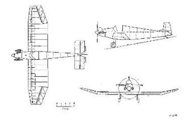
**Plans (drawings) for Sale:** \$250 (paid \$550) Karatoo J6C (Australian version of Karatoo). Larger, longer, 80hp to 100hp, steel tube fuselage, metal OR wood wing, folding wing option, removable rear cockpit tubing for use as camper vehicle. High wing and large windows for exceptional outside view. Luc Robillard Tel: 514-366-7500, cell: 514-298-3459
